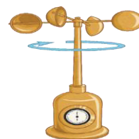
Anemometer Measures wind speed
