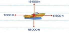
This boat is accelerating. The vertical forces have the same magnitude so their resultant is zero. The resultant force in the horizontal direction is 5500 - 1000 = 4500 N.
